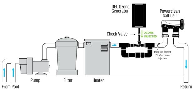
OZONE 25/50/100 WITH SALT SYSTEM & INJECTOR MANIFOLD KIT, (Ensure salt system is two feet from ozone generator)
