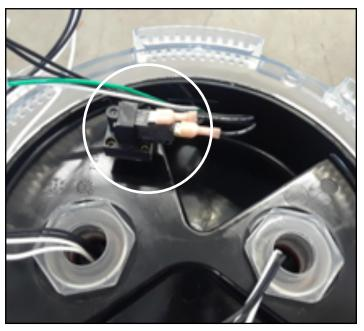
7. Locate pressure switch in the top of the DEL UV-C 50 main housing. **Do not remove the pressure switch, it will remain in place.**
