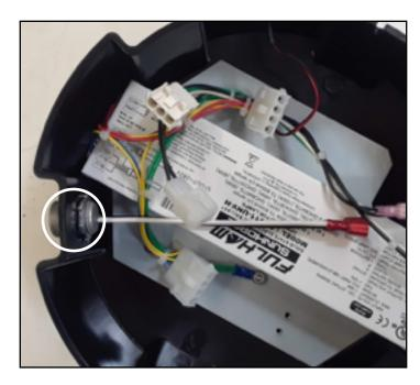
6. Remove nut from bulkhead connector. Route wiring through access cover hole and nut. Tighten nut to bulkhead connector. The bulkhead connector o-ring will form a water tight seal to the access cover.
