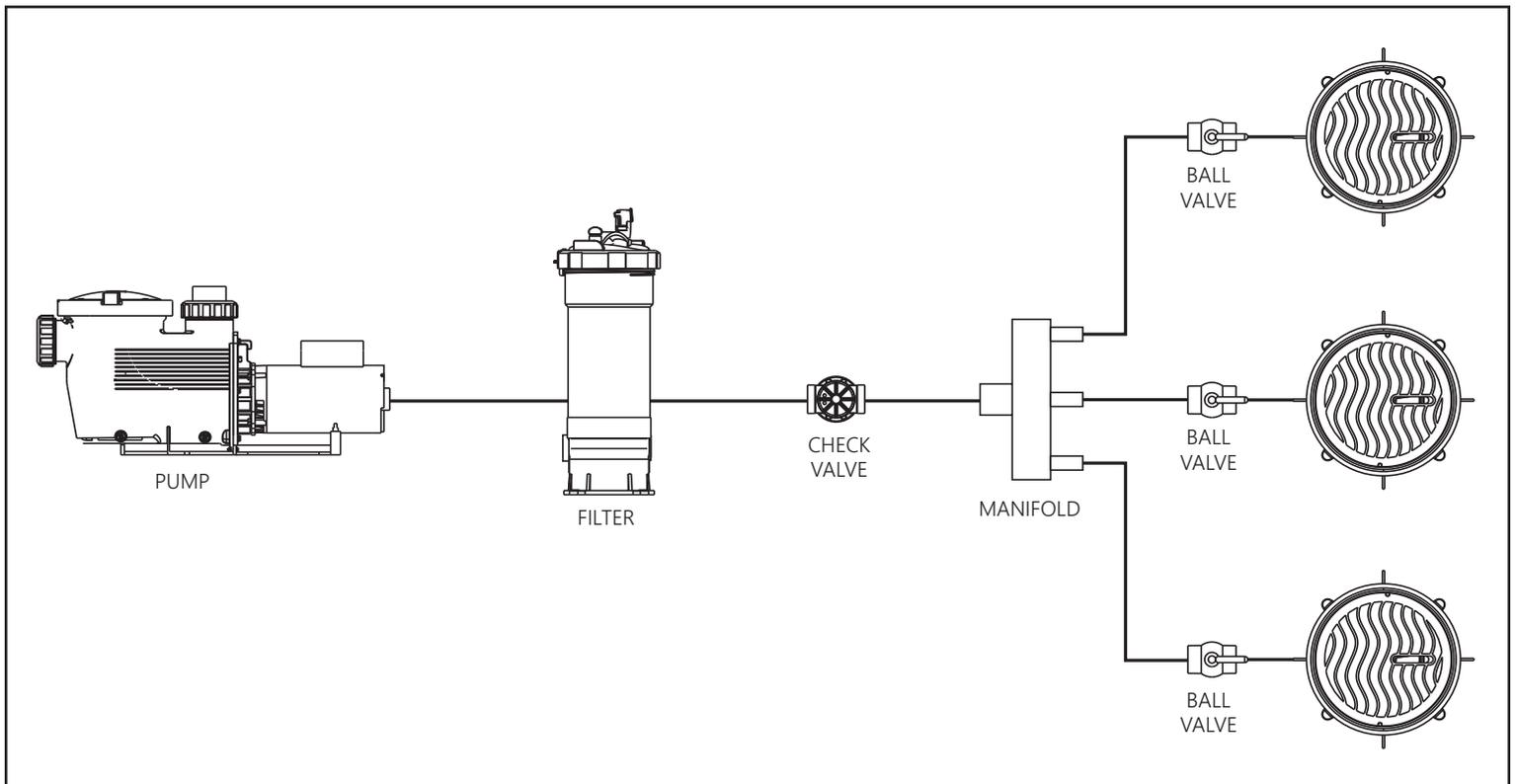
**FIGURE 3: SUGGESTED PLUMBING DIAGRAM FOR MULTIPLE Laminars**
