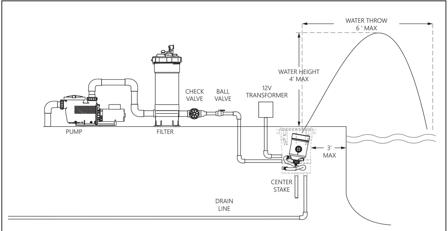
**FIGURE 2: SUGGESTED PLUMBING DIAGRAM FOR Laminars**
