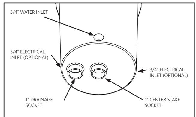
FIGURE 1: DECK CANISTER BOTTOM VIEW
